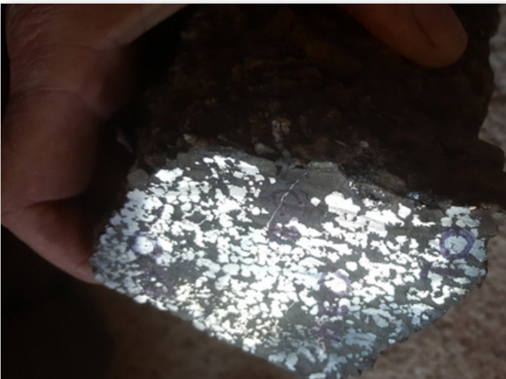
Figure 4. Cut through one of the silver nuggets showing the internal texture.
