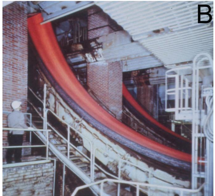
Figure 1. (A) Cross section of a continuous-casting machine for steel production (modified from Tselikov, 1984). (B) Photograph of continuously cast steel immediately following extrusion from the mold.
